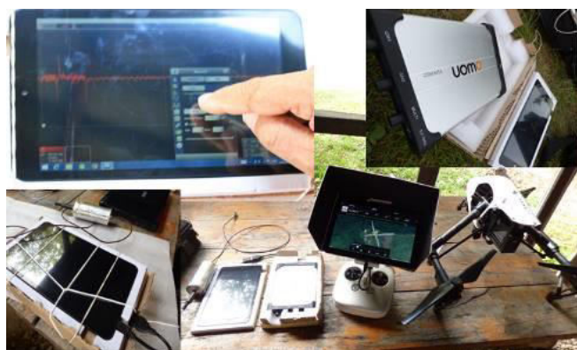
Slika 6, "Leteća laboratorija": VF-Broadband amplifier, special /light weight/, OBD LAB, Belgrade; PC osciloscop OWON, VDS1022; Tablet computer, I.Onik, Quad Core, Win 8.1
